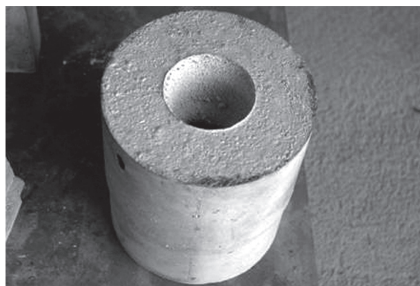
Figure 10. Pre-cast shape for using as burner pipe in cement kiln.
