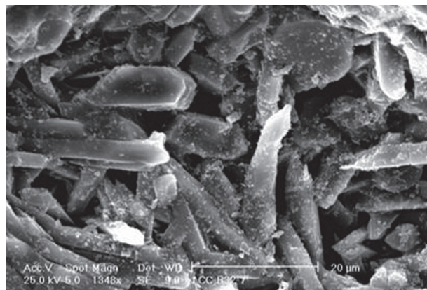
Figure 8. SEM photomicrograph of alumina castable containing PCE (FS 20) after firing at 1500°C.
