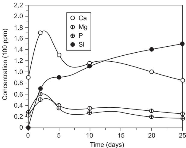
Figure 6. Variation of Ions concentration in SBF, in case of G1, with different soaking times.
