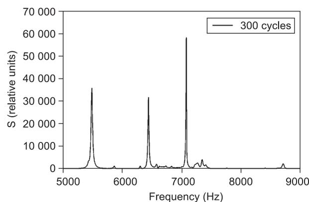
Figure 5. Response frequency spectrum, type 1 tile No. 305, after a series of 300 freeze-thaw cycles.
