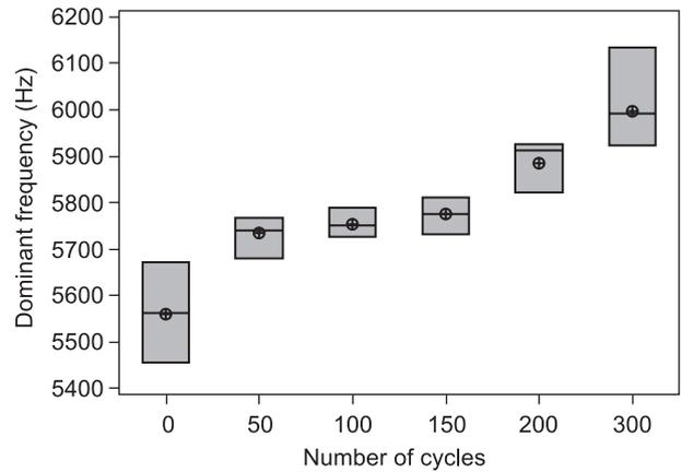
Figure 8. Dominant frequency occurrence regions and mean values, ⊕ versus the number of freeze-thaw cycles for type 2 tiles.
