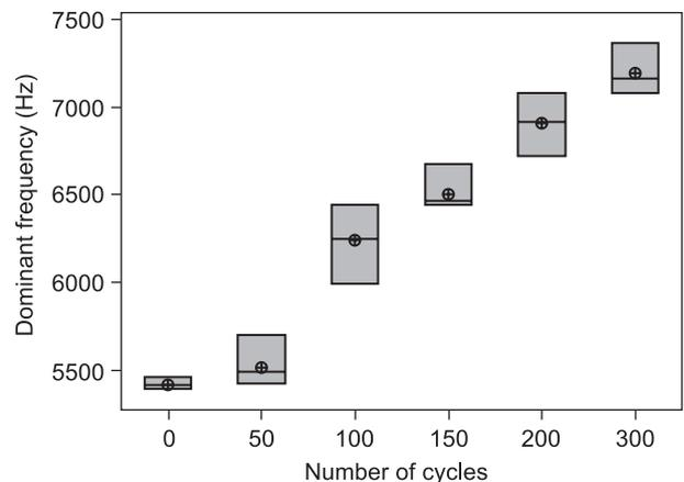
Figure 9. Dominant frequency occurrence regions and mean values, ⊕ versus the number of freeze-thaw cycles for type 3 tiles.
