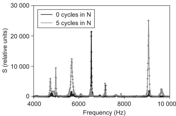
Figure 11. Shift of the dominant frequencies in type 2, No 41 specimen, in the course of 5 accelerated degradation tests with the temperature dropping down to - 70°C (0N - prior to, 5N - after five cycles).
