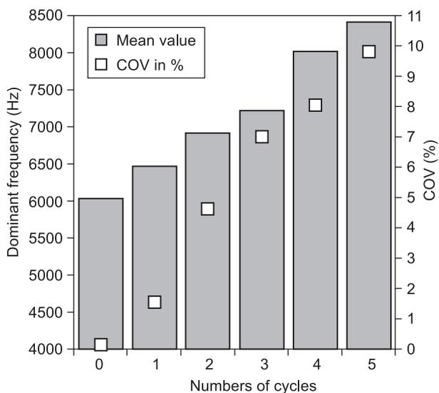
Figure 12. Mean values of the dominant frequencies and the corresponding variation coefficients for the different accelerated degradation stages for type 2 specimens.
