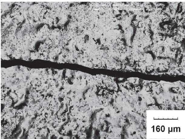
Figure 15. The crack after five accelerated stress cycles.
