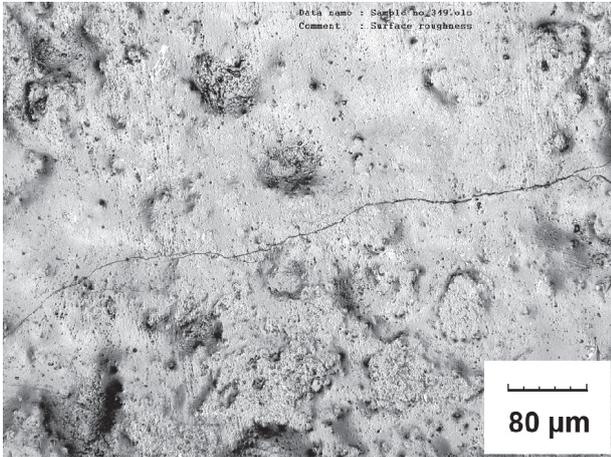
Figure 13. A fine crack which appeared after a single accelerated stress cycle.
