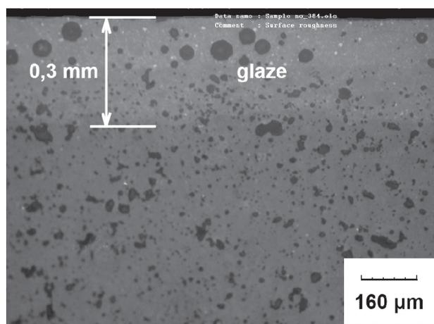
Figure 1. Section of type 1 ceramic tile.
