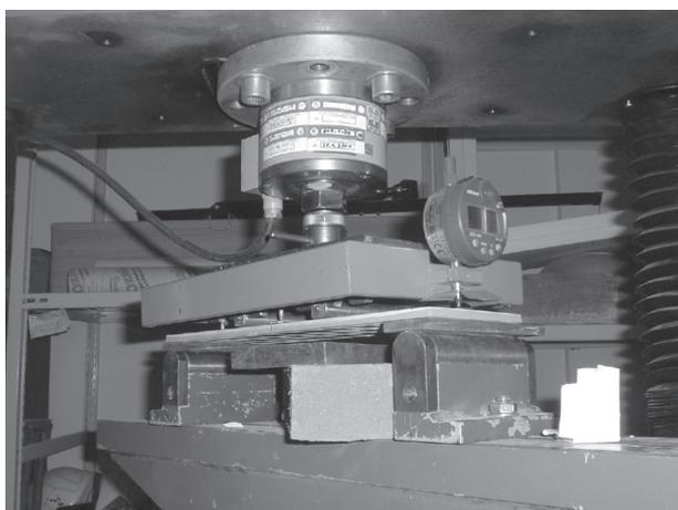
Figure 3. Specimen clamping detail.
