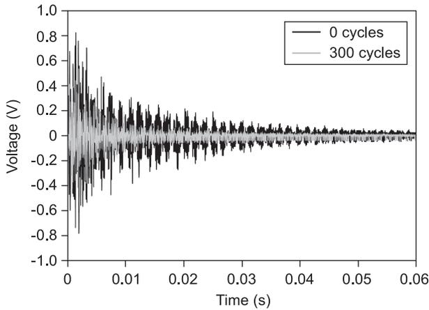
Figure 6. Time response record for type 1 tile No. 305, prior to and after 300 freeze-thaw cycles.
