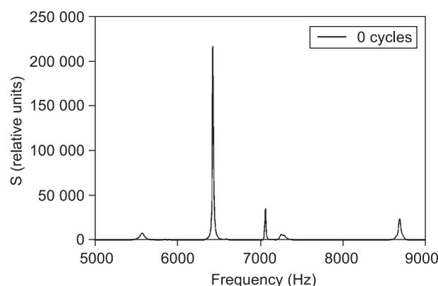
Figure 4. Response frequency spectrum, type 1 tile No. 305.
