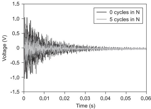
Figure 10. Time response for type 2 No 41 specimen prior to (0N) and after (5N) 5 accelerated degradation cycles.
