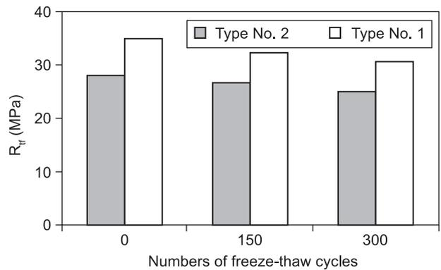
Figure 17. Cyclic-stressing induced strength variations for ceramic tiles.
