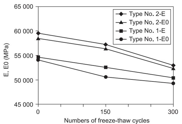
Figure 18. Cyclic-stressing-induced variations of the moduli of elasticity  $E$  and deformability  $E_0$  for ceramic tiles.
