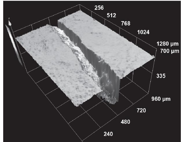
Figure 16. The crack relief for No. 41 tile after 5 accelerated degradation cycles.
