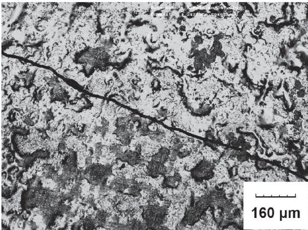
Figure 14. The same crack after three accelerated stress cycles.
