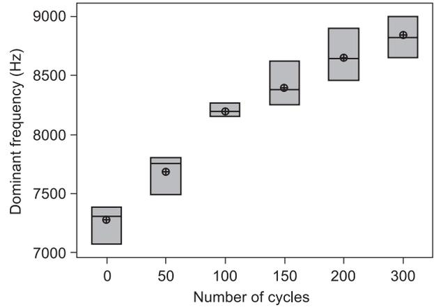
Figure 7. Dominant frequency occurrence regions and mean values, ⊕ versus the number of freeze-thaw cycles for type 1 tiles.
