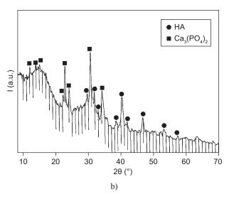
Figure 2. X-ray diffraction pattern of the HA coating: a) deposited by APS, b) after 21 days of immersion in SBF.
