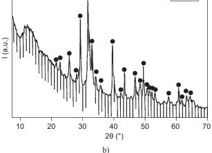
Figure 3. X-ray diffraction pattern of the HA coating: a) deposited by HVOF, b) after 21 days of immersion in SBF.
