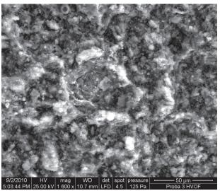
Figure 5. SEM image of as-sprayed HA coatings by HVOF.
