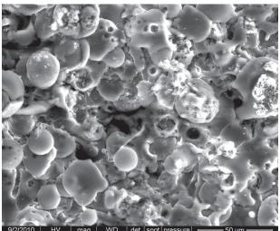
5.29.35 PM  $_{25.00 \text{ kV}}$  1 600 x 10.5 mm LFD 45 270 Proba 2P HA Figure 4. SEM image of as-sprayed HA coatings by APS.
