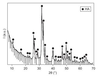
Figure 1. X-ray diffraction pattern of hydroxyapatite powder.
