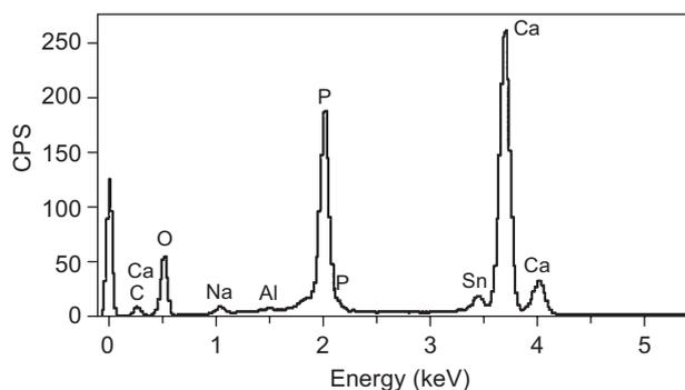
Figure 3. SEM EDAX data for hydroxyapatite exposed to  $\text{SnF}_2$  solution (1000 ppm with respect to fluoride) for 1 h showing small peak for tin at about 3.4 keV.
