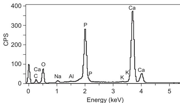
Figure 1. SEM EDAX data for as-received hydroxyapatite showing no peak for Sn.
