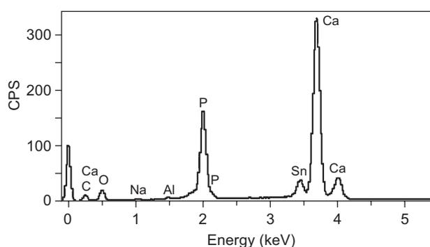
Figure 2. SEM EDAX data for hydroxyapatite exposed to  $\text{SnF}_2$  solution (500 ppm with respect to fluoride) for 1 h showing small peak for tin at about 3.4 keV.
