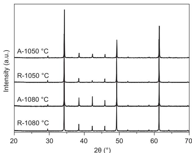
Figure 2. XRD profiles for different CCTO ceramics.
