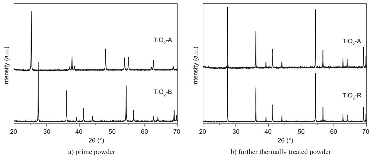
Figure 1. XRD profiles for different  $\text{TiO}_2$  raw materials.
