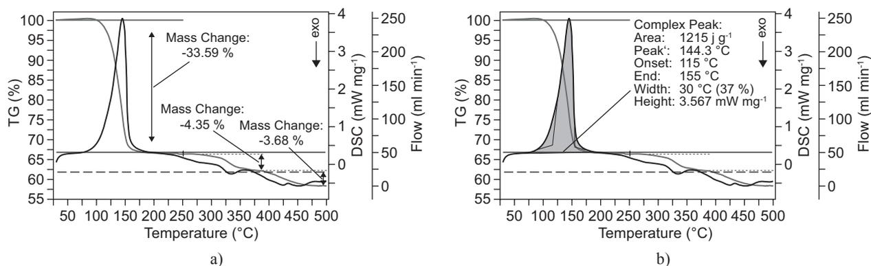
Figure 1. The thermoanalytical curves of thaumasite; a) evaluation of mass losses ( $\Delta m$  in %) on TG curve, b) evaluation of the decomposition enthalpy ( $\Delta H$  in  $\text{J g}^{-1}$ ) on DSC curve in the key decomposition step of 50–250°C.
