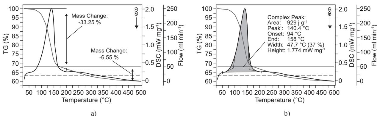
Figure 2. The thermoanalytical curves of ettringite; a) evaluation of mass losses ( $\Delta m$  in %) on TG curve, b) evaluation of the decomposition enthalpy ( $\Delta H$  in  $\text{J g}^{-1}$ ) on DSC curve in the key decomposition step of 50–250°C.
