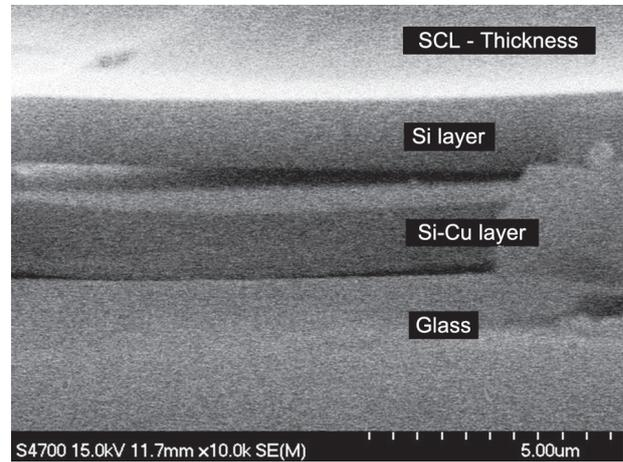
Figure 3. SEM/EDS cross-section of SCL coating.
