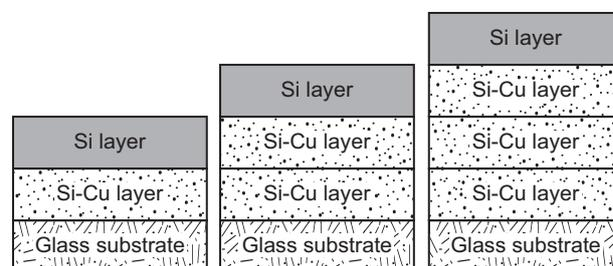
Figure 1. Multi-layer silica-copper coating on the glass substrate.
