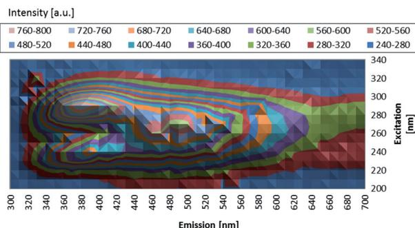
Figure 4. Example of luminescence spectrum of optical layer containing Cu<sup>+</sup> ions with 3 important maxims (SCP coating).
