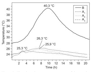
Figure 6. Time dependent temperature curves of the samples prepared by water  $(A_1-A_3)$  and by standard procedure (B).
