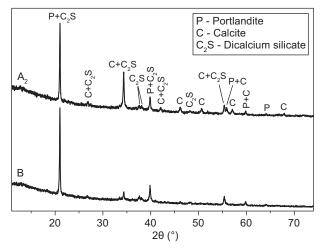
Figure 5. XRD pattern of sample prepared by water procedure  $(A_2)$  and of sample prepared by standard procedure (B) after 21 days of curing.
