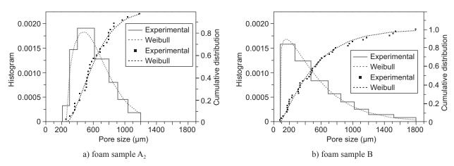
Figure 4. Pore size distribution of foam concrete prepared with the use of water procedure  $(A_2)$  and of foam concrete prepared by standard method (B).
