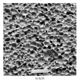
Figure 7. Microstructure of samples prepared without (B)/ with (A) applying of water procedure to the foams containing 30 % of origin cement content. Mixture sedimented in water for 3 min.
