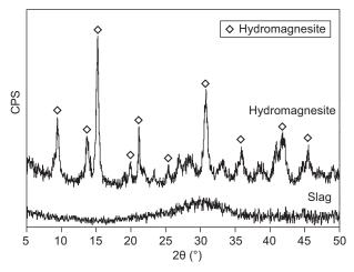
Figure 1. XRD pattern of hydromagnesite and slag samples.
