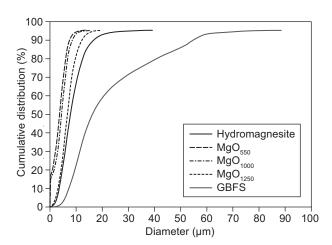
Figure 2. Particle sizes distribution of hydromagnesite and  $MgO_{550}, MgO_{1000}$  and  $MgO_{1250}$ .
