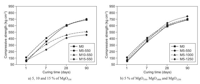
Figure 6. Compressive strength of AAS bleded with a) 5, 10 and 15 % of MgO<sub>550</sub> and b) 5 % of MgO<sub>550</sub>, MgO<sub>1000</sub> and MgO<sub>1250</sub>.
