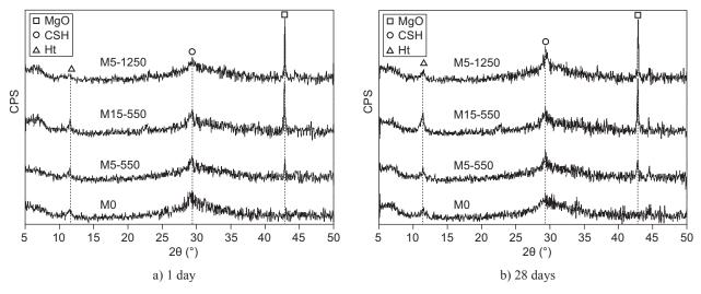
Figure 8. XRD diffractograms of reference specimens and AAS-MgO blends after a) 1 day and b) 28 days.
