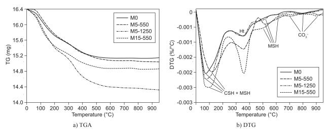
Figure 10. TGA (a) and DTG (b) of AAS and AAS-MgO blends after 28 days.
