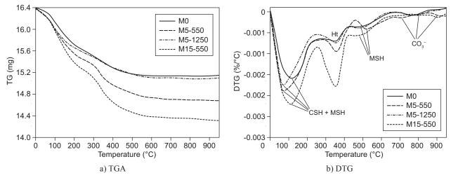
Figure 9. TGA (a) and DTG (b) of AAS and AAS-MgO blends after 1 days.
