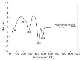
Figure 3. DTA thermogram of hydromagnesite.
