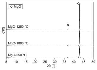
Figure 4. XRD pattern of MgO calcined at 550, 1000 and 1250°C.
