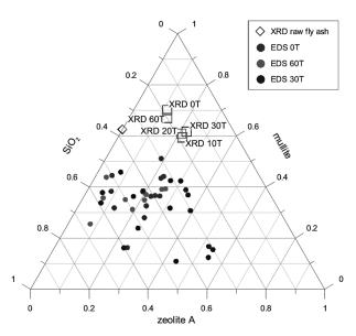
Figure 2a. Composition of EDS measurement points (dots) recalculated to three normative components: nepheline (dehydrated zeoliteA), mullite 2:1, quartz. Squares: reference bulk composition calculated based on crystalline phases from quantitative XRPD.
