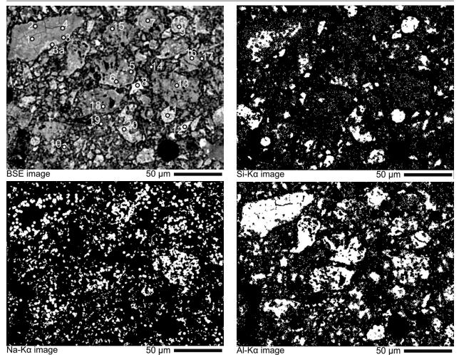
Figure 3a. BSE images with the measurement points and XRM images for sample 0T.
