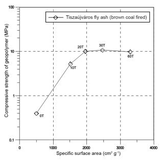
Figure 4b. Compressive strength of geopolymer as function of specific surface area of fly ash.
