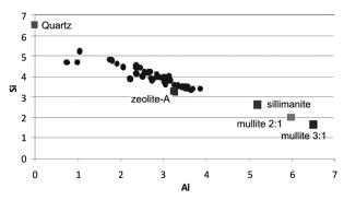
Figure 2b. Distribution of Si as a function of Al (dots) from chemical composition of EDS measurement points from samples 0T, 30T, 60T. All chemical compositions were recalculated for 13 oxygens. Squares: reference bulk composition of mineral phases identified by XRDP.
