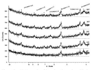
Figure 1b. XRPD graphs of investigated samples, with the peaks of zeolite-A phase magnified, note its absence in the geopolymer from unground and long time ground material (Z-A = zeolitye-A, STS = sodalite type structure, Q = quartz, Mu = mullite, Cc = calcite, ZnO = zincite).
