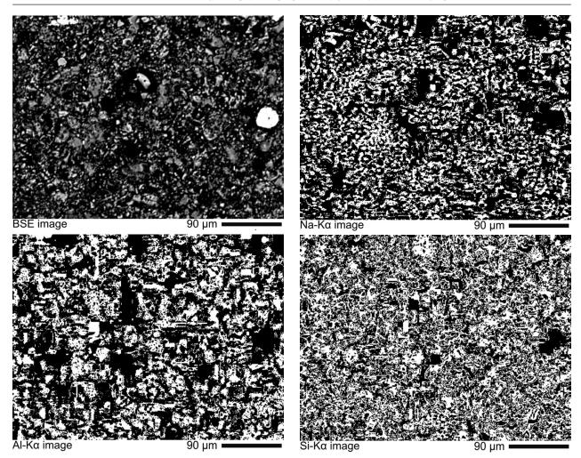
Figure 3b. BSE images with the measurement points and XRM images for sample 60T.
