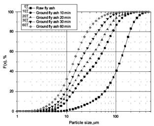
Figure 4a. Grain size distribution of ground fly ash material, before alkali-activation. Note the shift of distribution towards lower sizes, within the same range.
