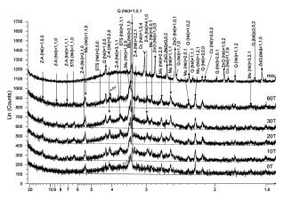
Figure 1a. XRPD graphs of investigated samples. Note the similar position for amorphous hump of glass (mix), geopolymer from unground fly ash (0T) and geopolymer samples (Z-A = zeolitye-A, STS = sodalite type structure, Q = quartz, Mu = mullite, Cc = calcite, ZnO = zincite).
