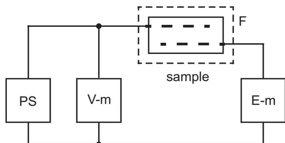
Figure 1. Basic scheme of the DC conductivity measurement; PS – stabilized power supply, V-m – voltmeter, E-m – electrometer, F – furnace.
