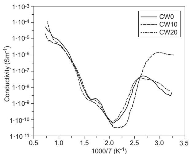
Figure 6. Temperature dependences of the DC conductivity for samples CW0, CW10 and CW20 on the reciprocal temperature.
