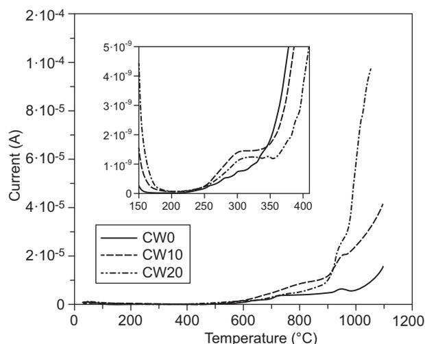
Figure 5. Temperature dependences of the DC current for samples CW0, CW10 and CW20. The inserted picture shows the temperature dependence of the DC current between 150°C and 400°C.
