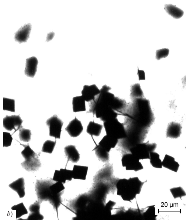
Figure 1. a) Spinel sludge in glass SS-AA; b) Spinel crystals bonded by RuO 2 needles [9].
