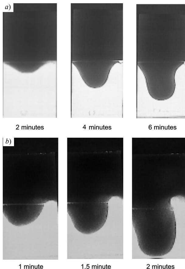
Figure 3. Motion of the interface between the liquid with suspended alumina particles ( $100 \mu\text{m}$ ) and the pure liquid. a)  $c = 12.5 \text{ kg m}^{-3}$ ; b)  $c = 25 \text{ kg m}^{-3}$
