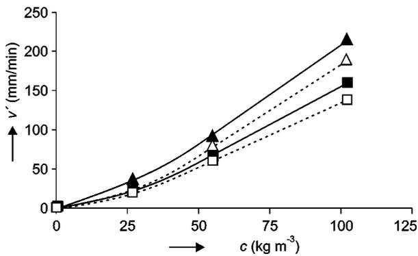
Figure 8. The comparison of experimental and calculated values of the settling front velocity.
