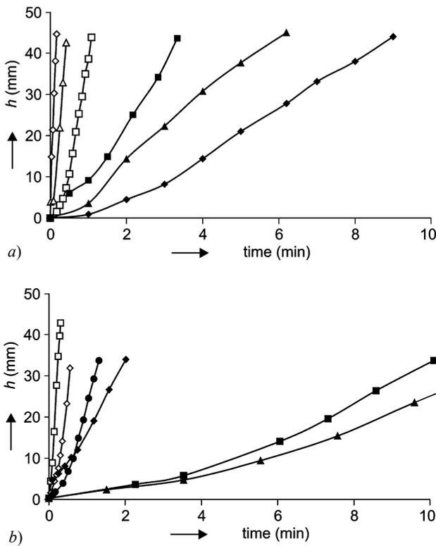
Figure 4. The shift of the settling front versus alumina particle concentration.
