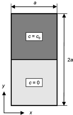
Figure 5. Initial and boundary conditions corresponding to the laboratory arrangement.
