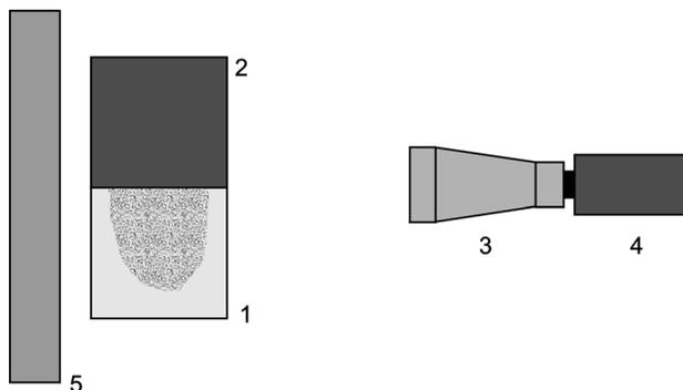
Figure 2. The scheme of the observation method: 1 - bottom cell with pure model liquid, 2 - upper cell with alumina suspension, 3 - objective, 4 - videocamera, 5 - illuminative box
