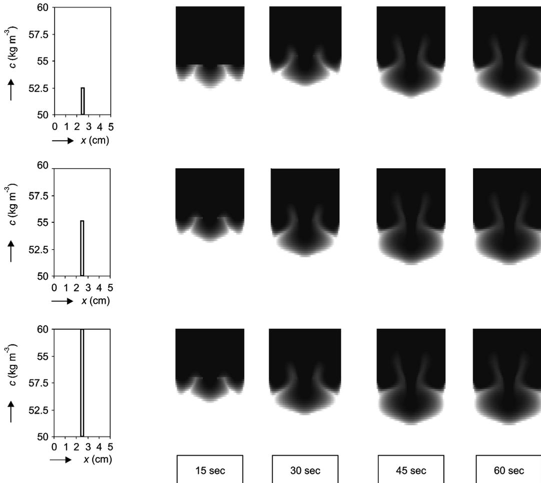
Figure 6. Calculated time developments of the settling front for different values of concentration fluctuation in the middle of the cell; the initial concentration of particles in the suspension was 50 kg m<sup>-3</sup>.
