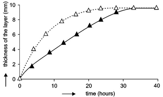
Figure 9. The experimental and calculated sedimentation rate of alumina particles ( $80 \mu\text{m}$ ,  $c = 100 \text{ kg m}^{-3}$ ).
