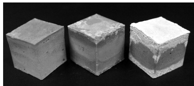
Figure 19. Specimens exhibiting no, slight, and severe efflorescence (from left).
