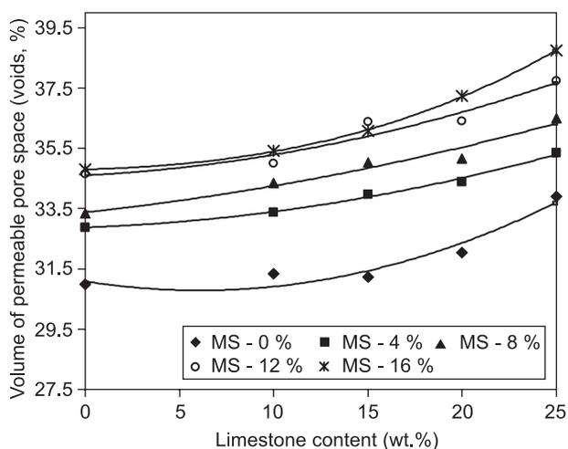
Figure 4. Volume of permeable space of cement pastes containing different proportions of microsilica and limestone powder.
