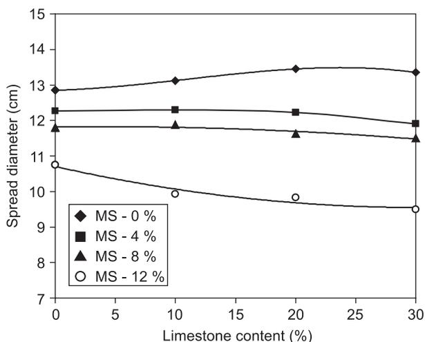
Figure 1. Spread diameter of cement pastes containing different proportions of microsilica and limestone powder.
