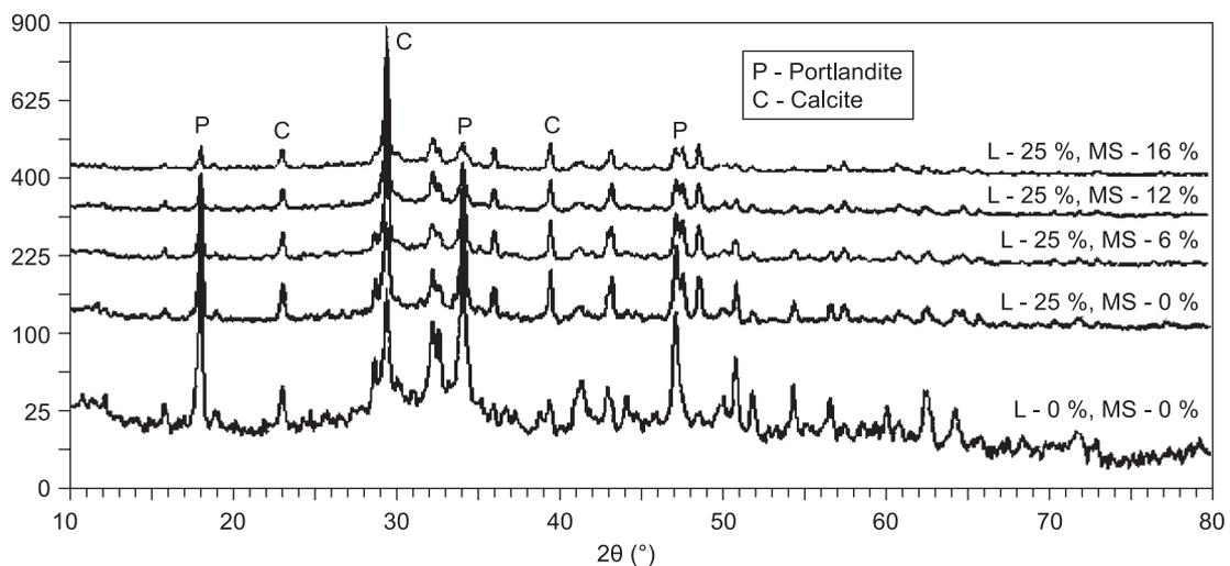
Figure 7. X-ray diffraction patterns of ternary blended cements containing different proportions of limestone powder and microsilica after 28 days of hydration.
