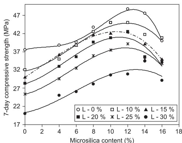
Figure 2. 7-day compressive strengths of ternary blended cements with limestone powder and microsilica.
