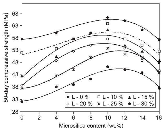
Figure 3. 50-day compressive strength of cement pastes containing different proportions of microsilica and limestone powder.
