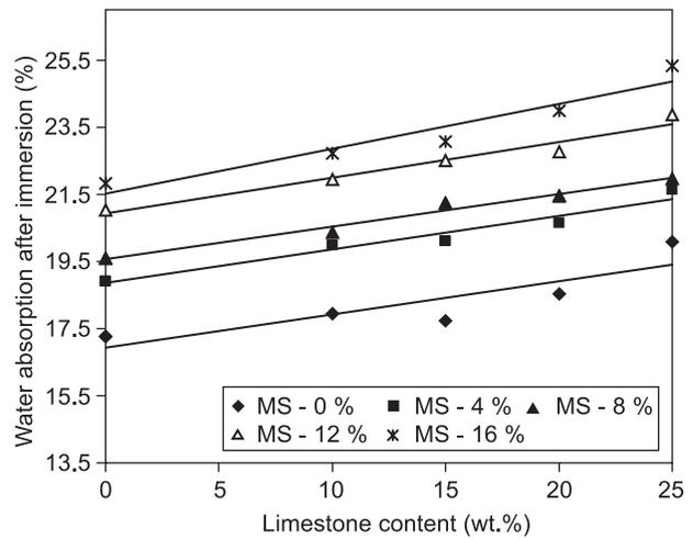
Figure 6. Water absorption of cement pastes containing different proportions of microsilica and limestone powder.
