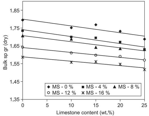
Figure 5. Bulk specific gravity of cement pastes containing different proportions of microsilica and limestone powder.
