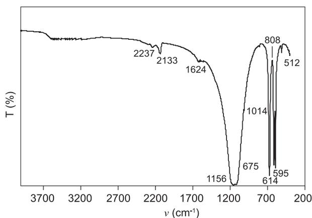
Figure 5. FT-IR spectrum of the anhydrite binder calcined at 800 and 900°C.
