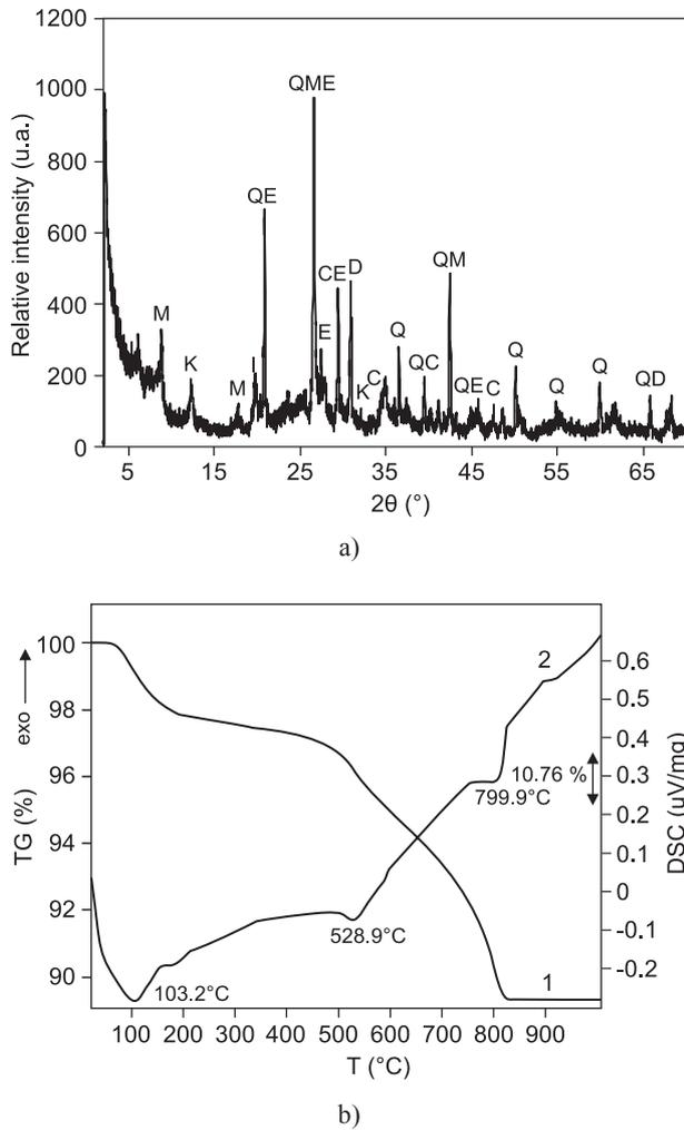
Figure 3. X-ray diffraction pattern (a) and STA curves (DSC - 1, TG - 2) (b) of the clay. (M - muscovite, K - kaolinite, I - illite, C - calcite, E - microcline, Q - quartz, D - dolomite).
