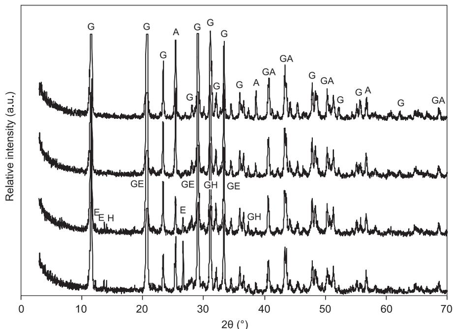
Figure 8. X-ray diffraction patterns of hydrated anhydrite binder: 1 - 1 mixture, 2 - 2, 3 mixtures, 3 - 4 mixture, 4 - 5 mixture. Composition of mixtures is reported in Table 1. Indexes: A - anhydrite  $\text{CaSO}_4$ ; G - gypsum  $\text{CaSO}_4 \cdot 2\text{H}_2\text{O}$ ; E - gismondite  $\text{CaAl}_2\text{Si}_2\text{O}_8 \cdot 4\text{H}_2\text{O}$ ; H - calcium aluminium silicate hydrate  $\text{Ca}_2\text{Al}_2\text{SiO}_7 \cdot 8\text{H}_2\text{O}$
