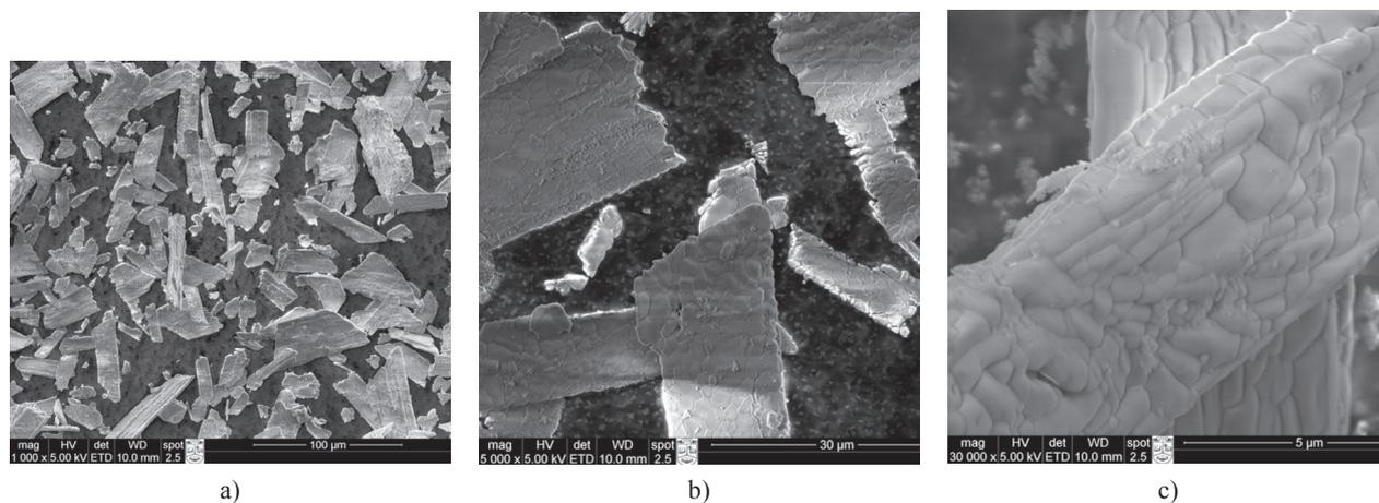
Figure 7. SEM microphotographs of anhydrite binder calcined at temperature 900°C: a, b, c - different magnification.
