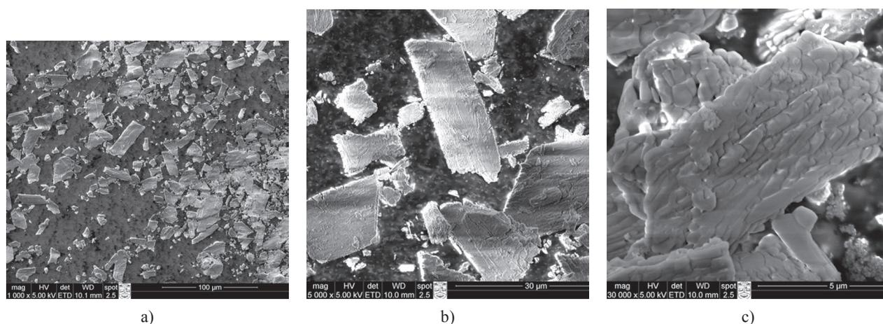
Figure 6. SEM microphotographs of anhydrite binder calcined at temperature 800°C: a, b, c - different magnification.
