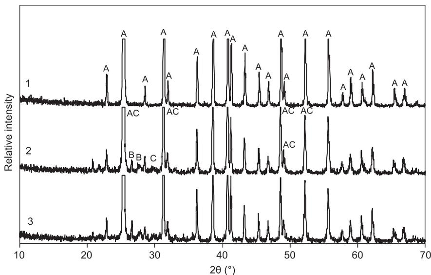
Figure 4. X-ray diffraction patterns of anhydrite binder calcined at 900 °C: 1 - 1, 2, 3 mixtures, 2-4 mixture, 3-5 mixture; composition of mixtures is reported in Table 1 (A - anhydrite CaSO<sub>4</sub>; B - anorthite CaAl<sub>2</sub>Si<sub>2</sub>O<sub>8</sub>-CAS<sub>2</sub>; C - gehlenite Ca<sub>2</sub>Al<sub>2</sub>SiO<sub>7</sub>-C<sub>2</sub>AS).
