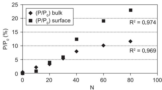
Figure 2. Damage of the samples ( $P/P_0$ ) during water quench test.
