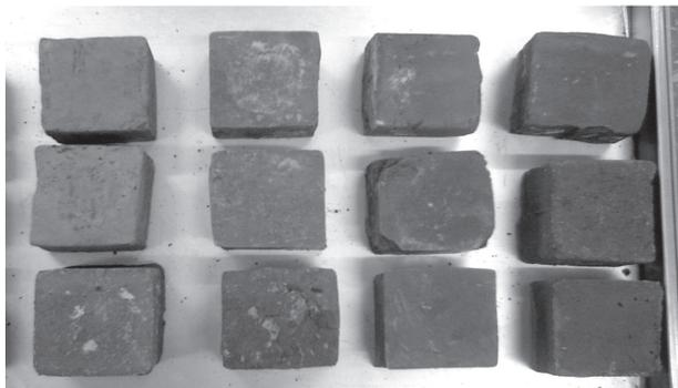
Figure 4. Solidified products developed from ELO, FA, P and C (after firing).
