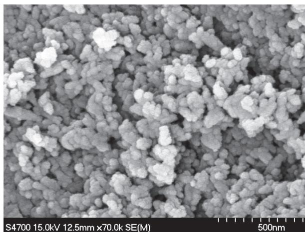
Figure 7. Surface of the original hydroxyapatite (HA) material before the exposure.
