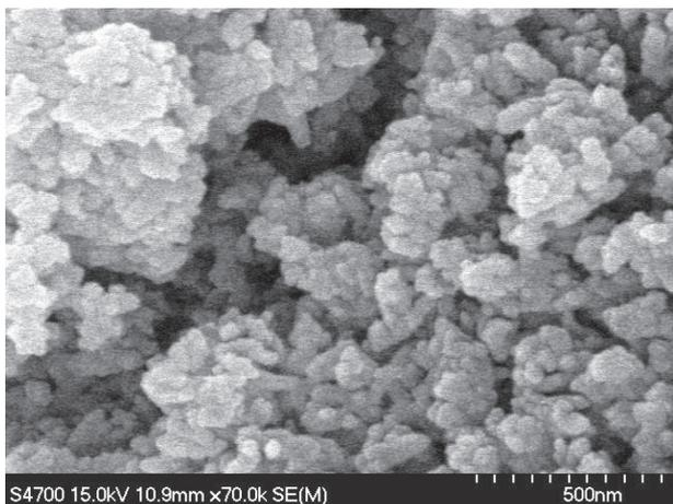
Figure 8. Surface of the  $\frac{1}{4}$ V HA material (from the partly filled testing cell) following the exposure to SBF.
