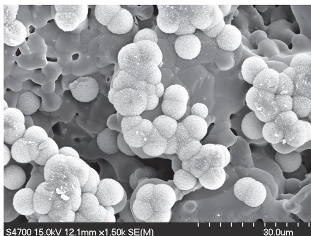
Figure 2. Surface of the material 1/4V TCP (partly filled testing cell) after the exposure to SBF with the newly formed HAp phase.
