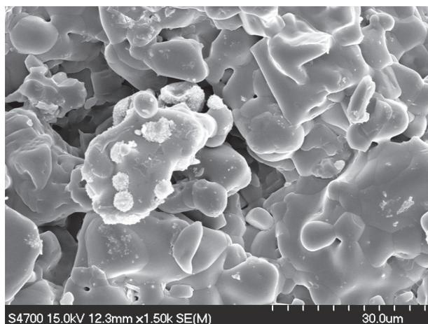
Figure 3. Surface of the 1V TCP material (completely filled testing cell) after the exposure to SBF.
