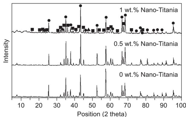
Figure 7. XRD results of refractory castables containing different amounts of nano-titania particles after firing at 1550°C (● - Corundum, ■ -  $CA_6$ , ▲ - Perovskite).
