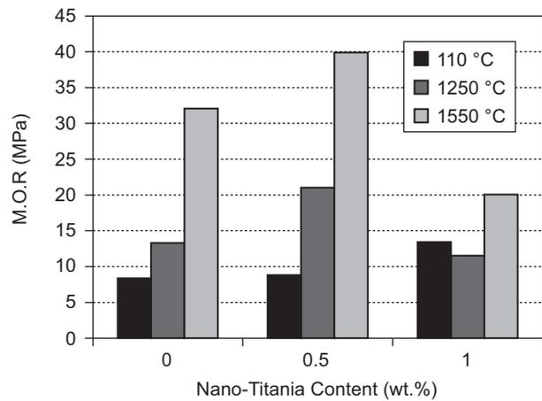
Figure 5. The effect of nano-titania content on the M.O.R. of refractory castable as a function of firing temperature.
