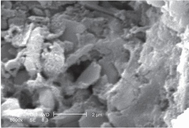
Figure 8. SEM photomicrograph of high-alumina refractory castable containing 0.5 wt. % nano-titania particles fired at 1250°C.
