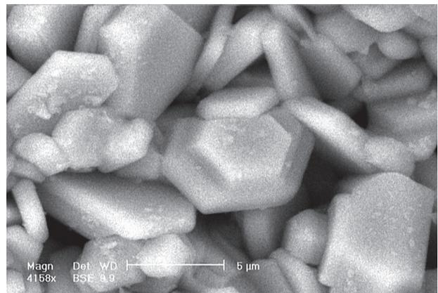
Figure 12. SEM photomicrograph of high-alumina refractory castable containing 1 wt.% nano-titania particles fired at 1550°C.
