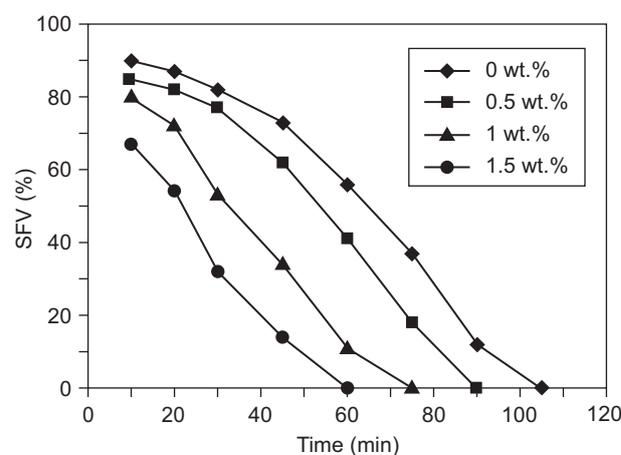
Figure 1. The effect of nano-titania content on SFV of refractory castable as a function of time.
