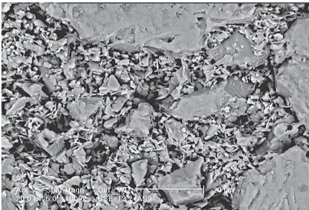
Figure 9. SEM photomicrograph of high-alumina refractory castable without nano-titania particles fired at 1550°C.
