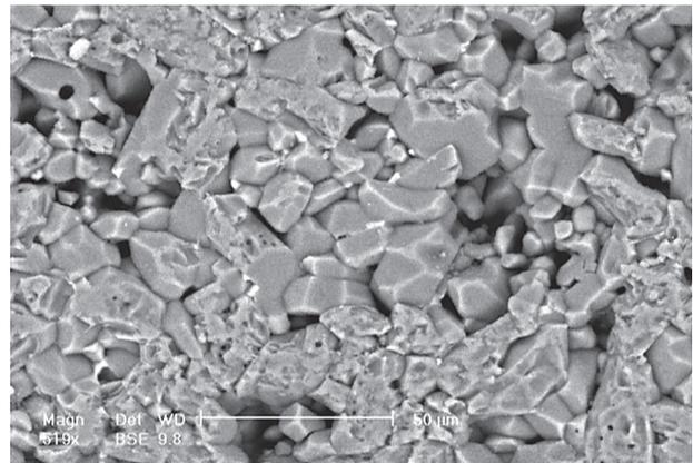
Figure 11. SEM photomicrograph of high-alumina refractory castable containing 1 wt.% nano-titania particles fired at 1550°C.
