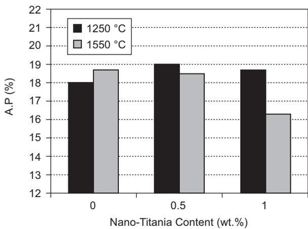
Figure 3. The effect of nano-titania content on the A.P. of refractory castable as a function of firing temperature.
