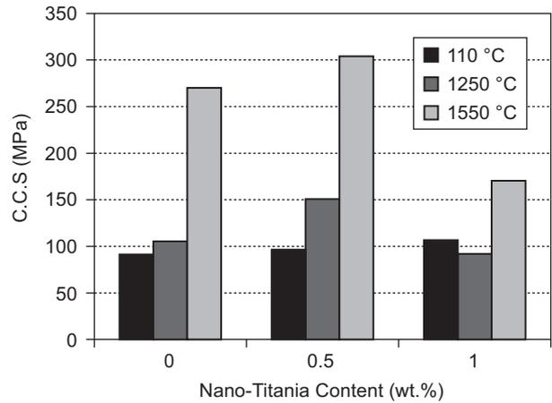
Figure 4. The effect of nano-titania content on the C.C.S. of refractory castable as a function of firing temperature.
