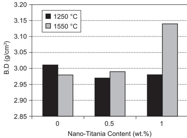
Figure 2. The effect of nano-titania content on the B.D. of refractory castable as a function of firing temperature.
