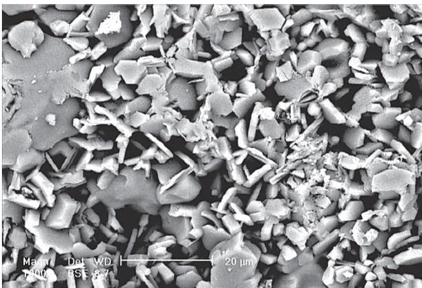
Figure 10. SEM photomicrograph of high-alumina refractory castable containing 0.5 wt.% nano-titania particles fired at 1550°C.
