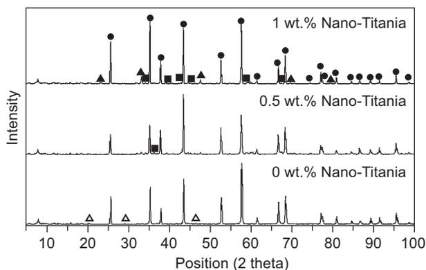
Figure 6. XRD results of refractory castable containing different amounts of nano-titania particles after firing at 1250°C (● - Corundum, ▲ -  $CA_2$ , ▲ - Perovskite, ■ -  $CA_6$ ).
