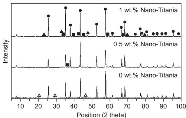
Figure 6. XRD results of refractory castable containing different amounts of nano-titania particles after firing at 1250°C (● - Corundum, Δ - CA<sub>2</sub>, ▲ - Perovskite, ■ - CA<sub>6</sub>).
