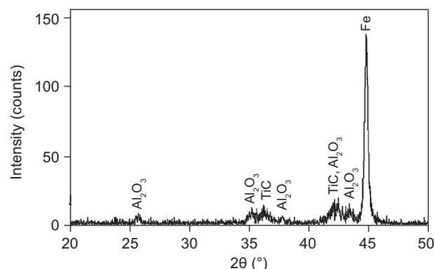
Figure 2. XRD pattern of the 80 h milled sample after annealing at 1000°C (stainless steel cup and balls).
