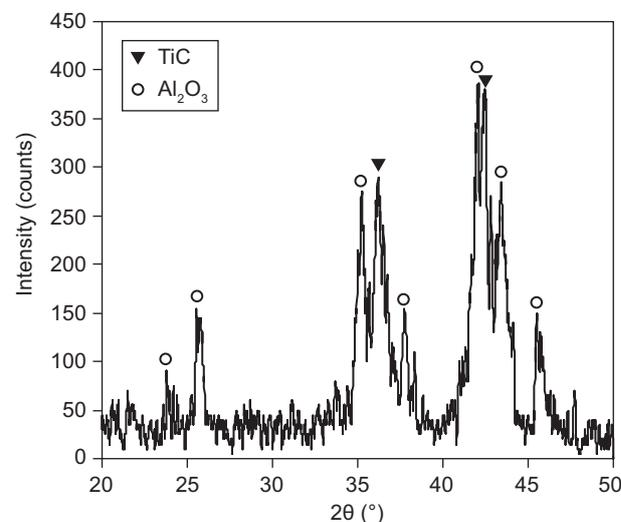
Figure 4. XRD pattern of the 35 h powder milled after leaching with 3HCl–HNO<sub>3</sub>.
