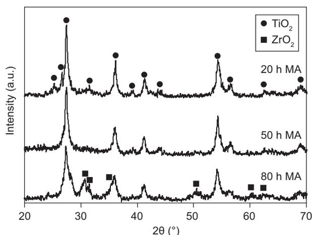
Figure 3. XRD pattern of the powders milled by ZrO<sub>2</sub> cup and balls.
