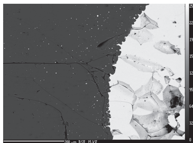
Figure 3. Irregular molybdenum corrosion in glass melt containing 1 % \text{Sb}_2\text{O}_3 , at current load of 1.5 \text{ A}\cdot\text{cm}^{-2} , with numerous metallic particles scattered in the glass (left).
