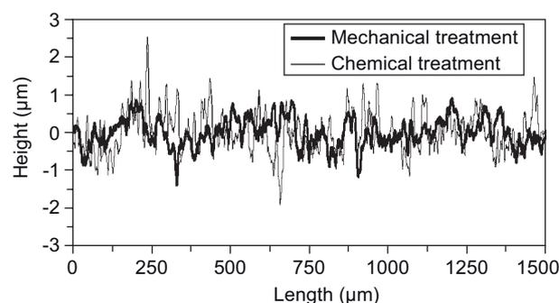
Figure 2. Profile comparison of Ti substrates after mechanical and chemical treatment.
