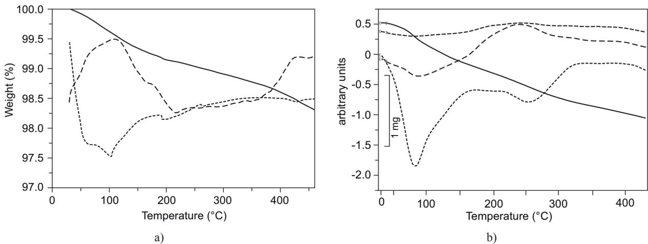
Figure 3. The representative TG, DTG and DTA curves of mechanochemically treated raw mixes for the duration of 1 minute (a) and 5 minutes (b).
