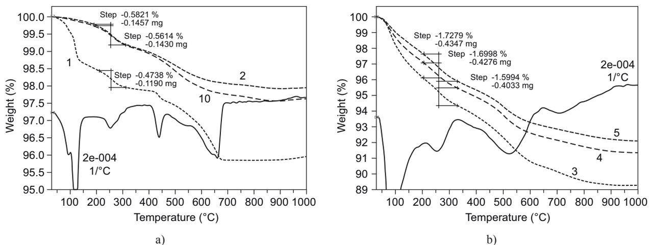
Figure 4. The evaluation of mass losses on TG curves in the temperature region 200-300°C which is sensitive on the presence (and thermal decomposition) of Al(Fe)-O-P cross-links; a) raw mixes mechanochemically treated for the duration of 5 minutes (in Table 3 referred as A. M., 5 min), b) final MDF probes [8, 9, 11] (in Table 3 referred as F. P.).
