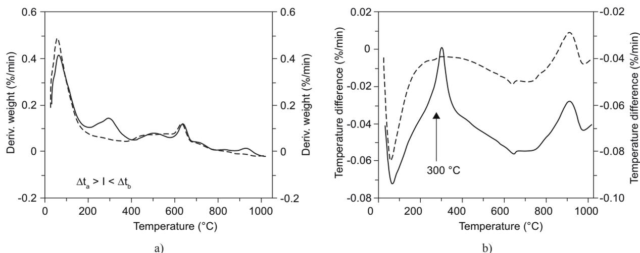
Figure 2. Typical DTG (a) and DTA (b) curves of MDF probes [8, 9, 11]; full lines with the events in the region from 200 to 300°C –  $\Delta t_b$  (DTG) and exoeffect at 300°C (DTA), denoting the occurrence of Al(Fe)–O–P cross-links (synthesis successful), dashed lines – no events in the region from 200 to 300°C due to the absence cross-links (synthesis not successful).
