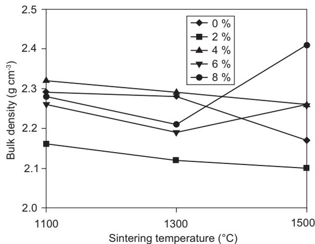
Figure 1. Bulk density of samples as a function of sintering temperature.
