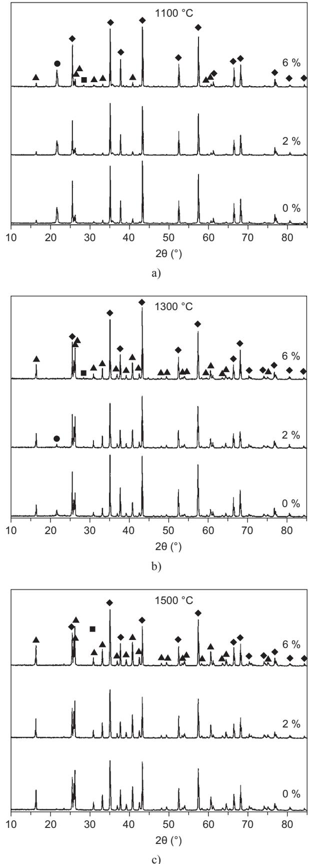
Figure 4. XRD patterns of specimens with different content of aluminum powder sintered at different temperature (● - SiO<sub>2</sub>, ◆ - Al<sub>2</sub>O<sub>3</sub>, ■ - Si, ▲ - mullite).
