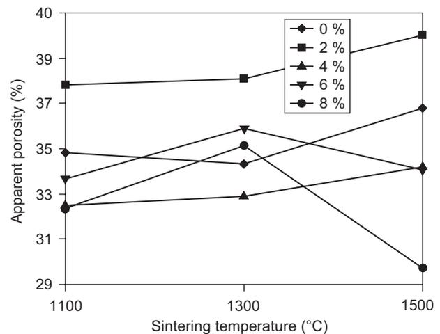
Figure 2. Apparent porosity of samples as a function of sintering temperature.
