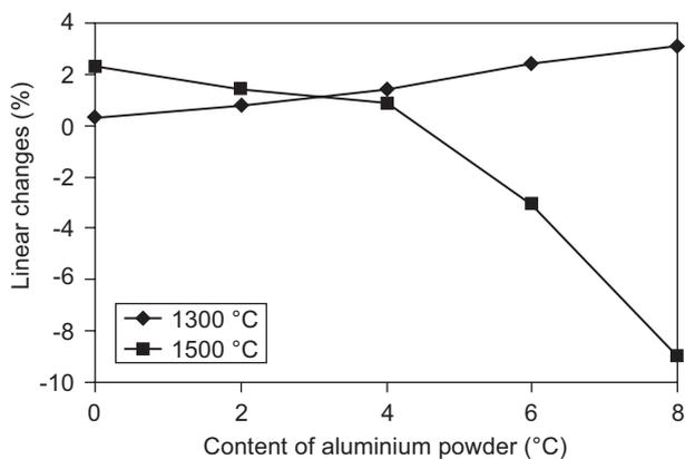
Figure 3. Linear changes in samples as a function of sintering temperature.
