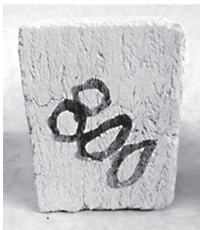
Figure 29. Cement foam immediately after firing at 800°C.
