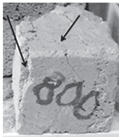
Figure 30. Cement foam fired at 800°C and kept one week in air (cracks).
