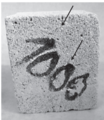
Figure 28. Cracks in the lime-silicate material after firing at 1000°C.
